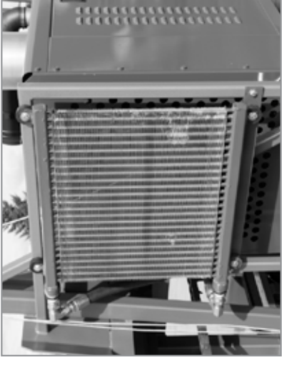
Hydraulic Oil Cooler
