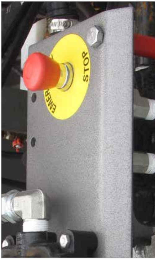
Emergency Shut Off Switch ("Panic Button")
